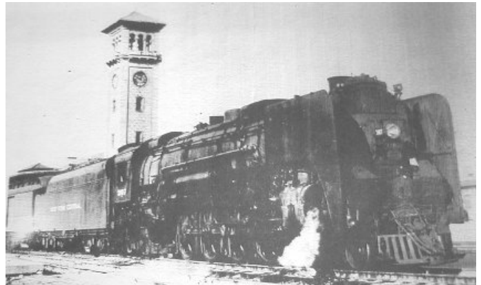
The New York Central designed the Mohawk (4-8-2) for fast freight service but as they grew older and traffic changed they proved to be very good with passenger trains. Here's the "Cleveland Special" about to leave Dayton in 1952.
